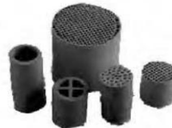
Carbon membrane supported on stainless steel
